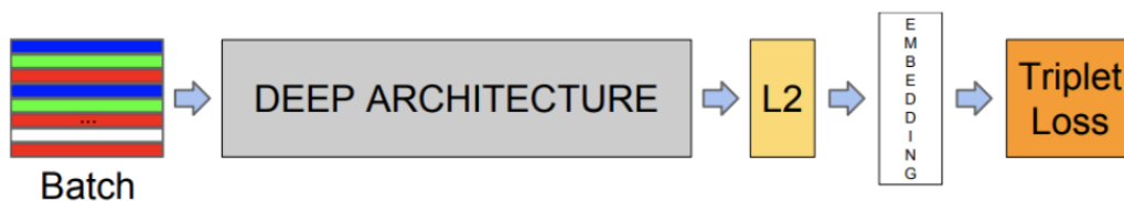
Figure 4: High Level Model Structure of Facenet
